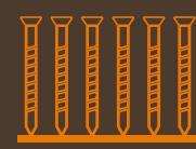
EXTERIOR RATED FASTENERS MIN #8 X 2 1/2" SCREWS OR MIN 8D X 2 1/2" RING SHANK NAILS
