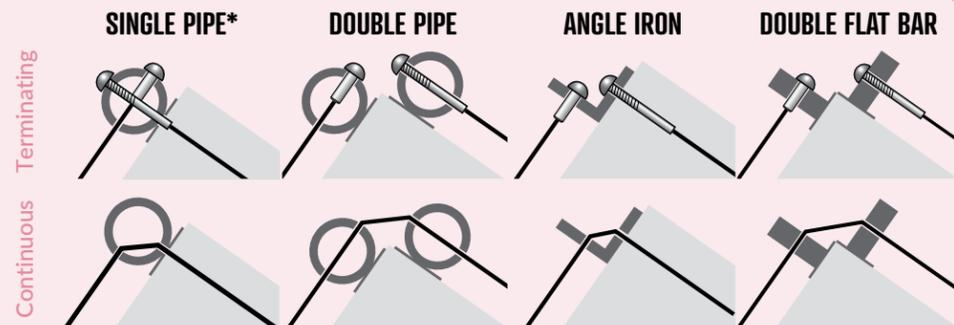
\*Offset drill holes at least 1/2" if you choose to have cables terminating at a single pipe post.
