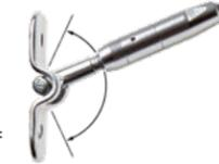
Fixed end fitting that attaches to the face of a post or wall with the included screws or bolts. 130° pivot range allows for angled stair terminations. Includes 2" lag screws for wood posts (3/8-in bolts for metal posts sold separately).
