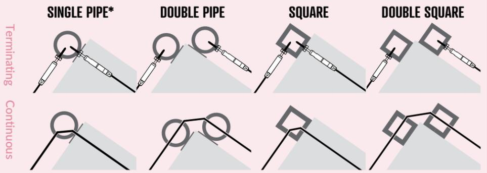
\*Offset drill holes at least 1/2" if you choose to have cables terminating at a single pipe post.
