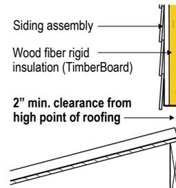
A 2 inch minimum clearance must be maintained between exterior TimberBoard siding assemblies where they meet roofs, decks, paths, steps, driveways or any other solid surfaces.
