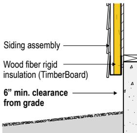
A 6 inch minimum clearance must be maintained between exterior TimberBoard siding assemblies and the ground.
