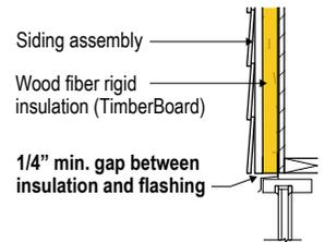
A 1/4 inch minimum clearance is necessary between exterior TimberBoard assemblies and any horizontal flashing. Ensure that all horizontal flashing is positioned with a positive slope to encourage effective drainage and prevent trapping of bulk water.
