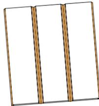
Apply a small bead of Cellular PVC adhesive to the bead/groove corner joints and grooved female ends of the three panel column wrap.
