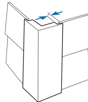
Fasten both sides according to standard AZEK Trim Guidelines. 4" Cornerboards may be installed using 2 fasteners at ends and splices and 1 fastener 12" OC through length of board.
