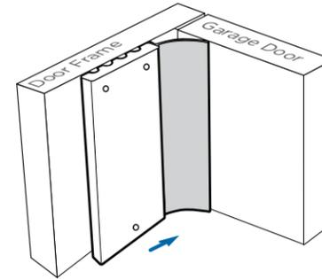
Firmly push Thermostop against Garage Door and fasten. Rubber seal should be in contact with Garage Door, but not overly tight. Place 2 fasteners within 1/2" of all ends and splices. All other fasteners should be 8" on center entire length of board.
