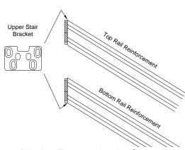
Attach an upper stair bracket to the angle cut end of the top rail reinforcement, with the bracket flush with the top of the reinforcement, using four *rail bracket screw* (A). Attach an upper stair bracket to the angle cut end of the bottom rail reinforcement, with the bracket flush with the bottom of the reinforcement, using four *rail bracket screw* (A). Lubricate the threads with soap to avoid binding and use a clutch type drill to avoid stripping screws.
