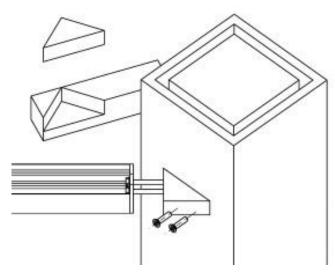
• This method is also used for radius rail attachment to newels, but using the radius rail brackets.
