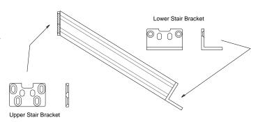
**b.** Measure and cut the upper end of both reinforcements to the rail angle determined in Step 1, include the protruding portion of the lower bracket as part of the total length.
