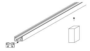
**c.** Locate crush block(s) provided to the bottom Aluminum Rail Reinforcement, with spacing no greater than 36" from the end, or between Crush Blocks.
