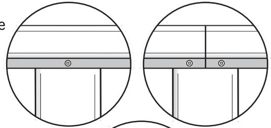
**4) Fasten Top Rails:** Secure the top rail to each post using two H screws (four screws for butt splices); screws should run through the cap rail flange and into the center of the post face. Attach screws to both the front and back of each post.
