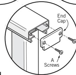
**5) Attach Decorative End Caps:** Attach the decorative end caps to all of the exposed top rail ends using two A screws. This applies to 200, 300, 350, and 450 Top Rail options.
