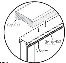
**5A) Cut & Attach Wood/Composite Cap Rails (for Series-450 Top Rails only):**
