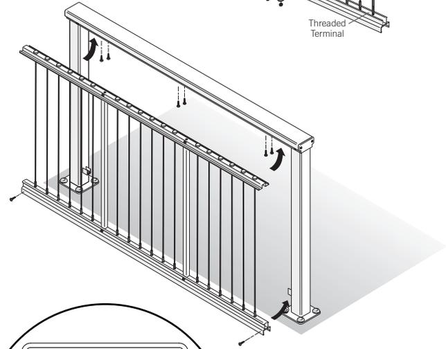
**13) Secure Panels:** Screw the top rail insert into the top rail from underneath with six "1" screws per panel, two on each end, two in center. Install bottom rails to RCBs with H screws.
