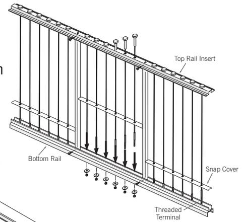
**12) Install Panels:** Place the assembled panel between posts and lift up into opening of the underside of the top rail. Make sure the RCBs fit into the upper channel of the bottom rail below the snap cover. Snap the top rail insert into the top rail once the infill is aligned.
