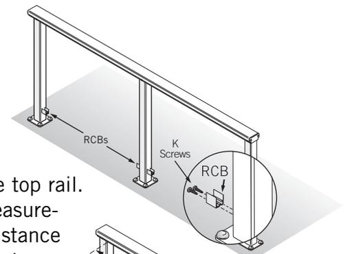
**7) Cut Top Rail Inserts:** Measure between each set of posts just below the top rail. Cut the top rail insert for each section to  $-1/16$ " of your corresponding measurement. Do not attach the top rail inserts to the top rail at this time. The distance between post and cable holes should be between 1-1/2" and 3" inches and equal on both ends. Standard configurations have 6 cables between posts and pickets. Number of cables and pickets may vary due to panel size. Consult your layout sheet.
