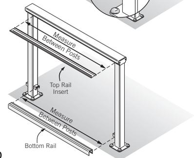
**8) Cut Bottom Rails:** Measure between each set of posts just above the RCBs. Cut the bottom rail for each section to  $-1/16$ " of your corresponding measurement. Make sure the holes in the bottom rail are in similar placement to the top rail insert so the cables run plumb vertically. Do not attach the bottom rails to the frame at this time.
