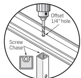
**11) Attach Pickets To Top Rail Insert:** Identify which end is the top end of each picket by comparing the spacing of the first cable hole in each picket to that of the first (top) pre-drilled cable hole on the posts. Use the F screws to attach the top end of the picket(s) to the top rail insert. **(If not using a bottom rails then skip to step 14).**
