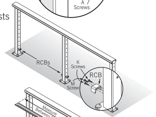
**8) Cut Bottom Rails:** Measure between each set of posts just above the RCBs. Cut the bottom rail for each section to  $+0/-1/16''$  of your corresponding measurement. Do not attach the bottom rails to the frame at this time.
