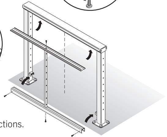
**14) Install Assembled Picket Panels Using Picket Base Plate Receiver:**
