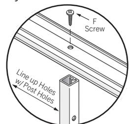
**12) Attach Pickets To Bottom Rail:** Using the F screws attach the bottom end of the picket(s) to the bottom rail. Assemble all sections using the same procedure.
