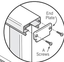
**7) Attach RCBs:** If using a bottom rail, locate the rail connecting bracket (RCB) holes on each post (these are pre-drilled except on stair rail posts where all the holes must be drilled in the field). Attach the RCBs to the posts using 2 K screws (outside holes) and 1 M screw (center position). The RCBs should be mounted wings down for frames using cable systems.
