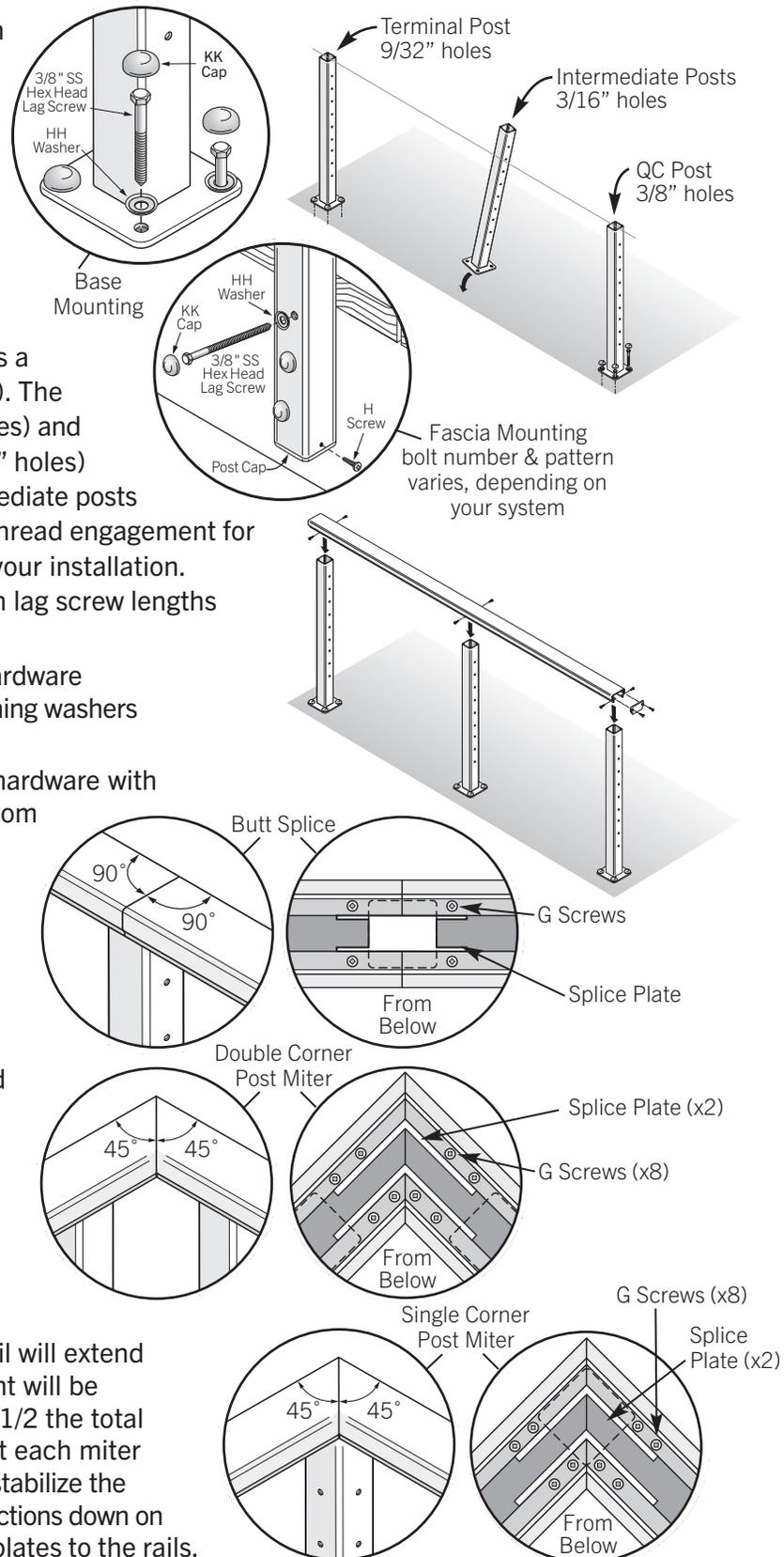
**5) Fasten Top Rails:** Secure the top rail to each post using two H screws (four screws for butt splices); screws should run through the top rail flange and into the post face. Attach screws to both the front and back of each post.
